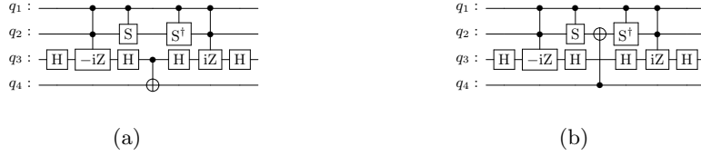
Fig. 5: A pair of Toffoli gates and an intermediate CNOT gate operating on the (a) target and (b) control qubits of the Toffoli gates.
